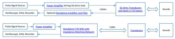
Wiring Information of Transmitting Sounds of a Transducer with T/R Switch.
