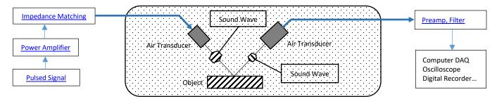
Pulse-Transmission System: Information Transmission through Air, Airlike Fluids, and DUT (Device Under Test).
