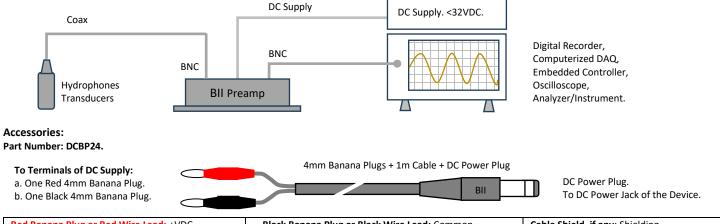
Red Banana Plug or Red Wire Lead: +VDC.
