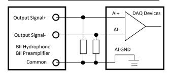
BII's Single-Ended Output to Single-Ended Input of a DAQ
