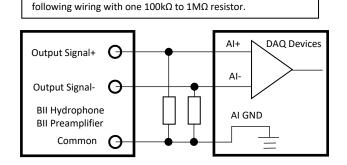
If input impedance of a DAQ device is greater than  $100M\Omega$ , use
