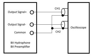
BII's Differential Output to Differential Input of a DAQ
