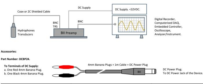
Red Banana Plug or Red Wire Lead: +VDC.
