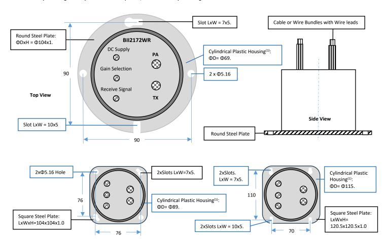
Note: (1) Height and Diameter of Cylindrical Plastic Housing and Round or Square Steel Chassis are determined by power rating.
