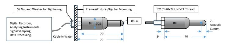
5. Free-hanging with Underwater Connector FHUWC-4P, 4 Pins (Fixed Sensitivity); FHUWC-6P, 6 Pins (Programmable Sensitivity).
