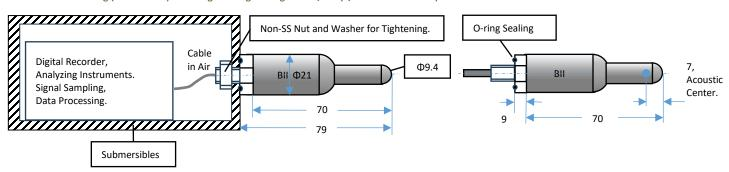
4. Bolt-Fastening Mounting BFM-7/16" (7/16"-20x22 UNF-2A).
