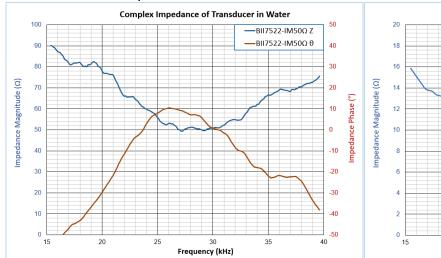
BII7522-IM6Ω Transducer Impedance:
