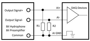
BII's Single-Ended Output to Differential Input of a DAQ
