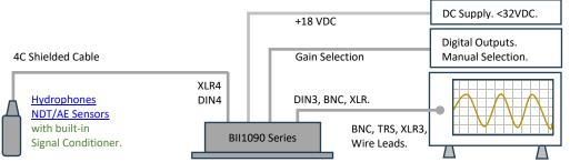
Digital Recorder, Computerized DAQ, Embedded Controller, Oscilloscope, Analyzer/Instrument.
