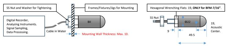
4. Thru-hole Mounting (Inch Thread) with Single O-ring Sealing THM-7/16" (7/16"-20x22 UNF-2A).
