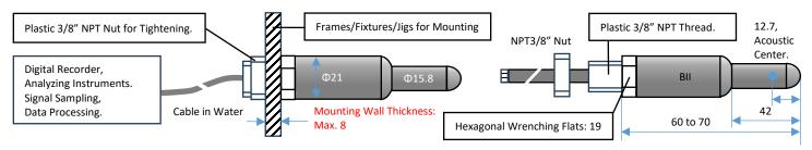
3. Bolt-Fastening Mounting BFM-7/16" (7/16"-20x22 UNF-2A), and BFM-5/8" (5/8"-18x22 UNF-2A, BFM-5/8" does NOT possess Hexagonal Wrenching Flats.).
