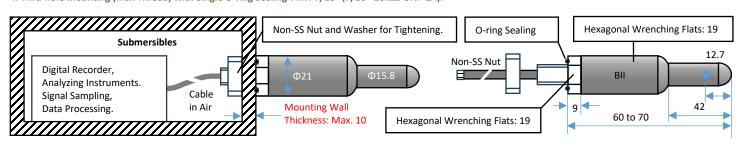
5. Free-hanging with Underwater Connector FHUWC-4P, 4 Pins (Fixed Sensitivity); FHUWC-6P, 6 Pins (Programmable Sensitivity).
