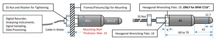
4. Thru-hole Mounting (Inch Thread) with Single O-ring Sealing THM-7/16" (7/16"-20x22 UNF-2A).
