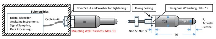
5. Free-hanging with Underwater Connector FHUWC-4P, 4 Pins (Fixed Sensitivity); FHUWC-6P, 6 Pins (Programmable Sensitivity).
