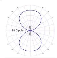
Cardioid Pattern= Omnidirectional Hydrophone + Dipole.
